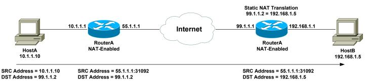
The above example demonstrates how the source (SRC) and destination (DST) IP addresses within the Network-Layer header are translated by NAT.
