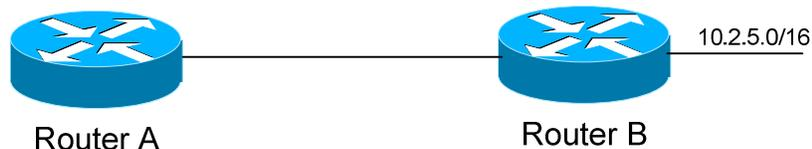
If Router B sends a routing update to Router A, it will *not* include the subnet mask for the 10.2.0.0 network. Thus, Router A must make a decision.
